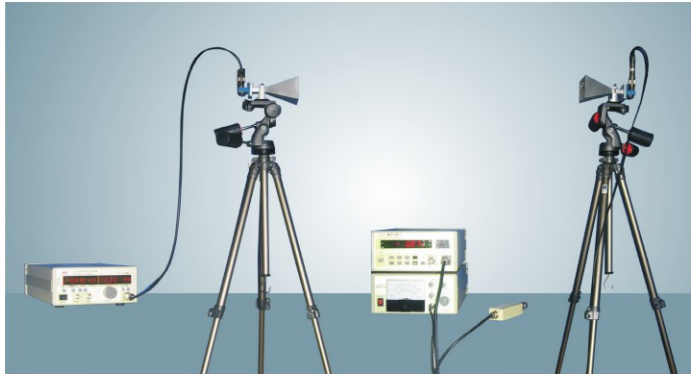
AT1123 standard signal generator (or AT1125 Gunn Oscillator, AT8201 Power Supply, AT8202 Function Generator and AT8341 PIN Modulator) AT2421 (AT437C) power meter (or TJ8-4 detector and AT3892 selective amplifier) are used to test direction of antenna to drawing direction diagram.
