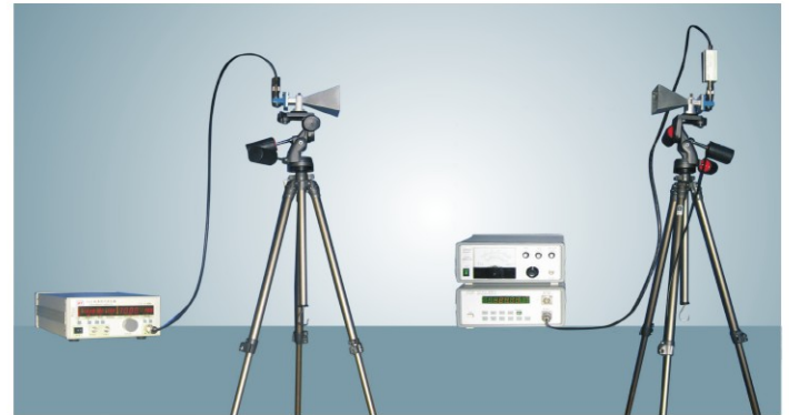
AT1123 standard signal generator (or AT1125 Gunn Oscillator, AT8201 Power Supply), AT2422 (or AT4373) power meter are used to test the direction of antenna.
